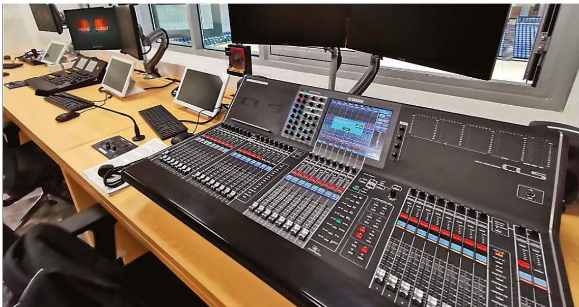
A Yamaha CL5 and MA Lighting MA2 onPC control the audio and lighting respectively
